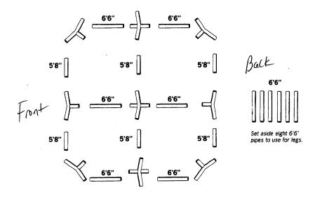
Connect pipes together starting with the center frame. Then assemble each side.
