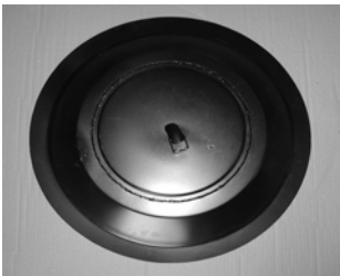
Figure 1D – Natural Gas Orifice
