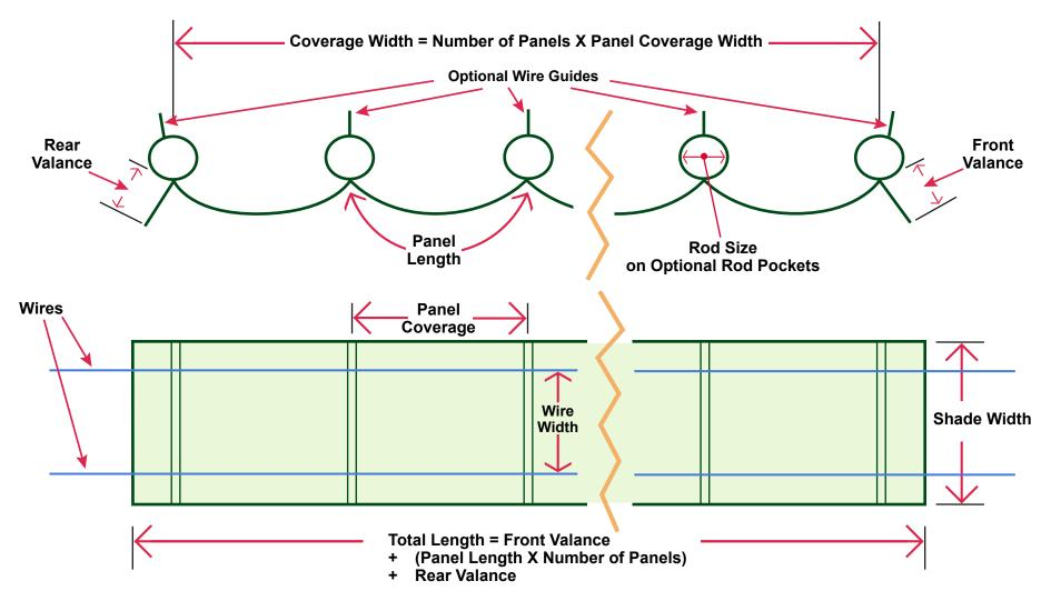
**VALANCE** - It's the fabric that extends from either end of the retractable slide wire canopy. Most times it is 1.5" and will have grommets for fastening to hold in place. It can be longer to provide additional shade from a rising or setting sun when near the horizon.
