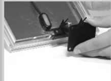
Fixing the Panel Holder
