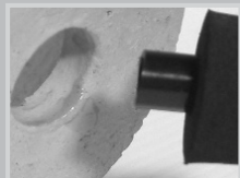
The hose and the rubber bung fits into the hole in the bottom of the jug
