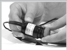
Remove pump base
