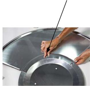
Next, align the sides of each outer piece and the center piece and insert the next 3 bolts through both holes. Tighten castle nuts on bolts.
