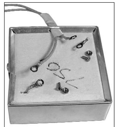
Figure 10 - Lead wires disconnected from element.
