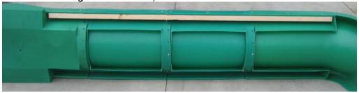
There are 8 - # 14 x 1 1/2" pan head screws. Three screws go in each side of the insert. Make sure the inserts are aligned and gaps are closed before the screws are inserted. Start at one end where the two sections meet together. Screw in the screw closest to the edges of the sections, then put the middle screw in the side. Add another section, making sure that it is aligned before inserting the screw. Make sure the screws are screwed into the wood straight and not crooked.
