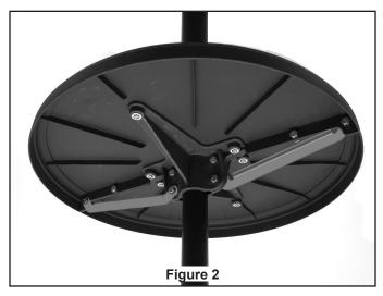
**2.** Fasten the table halves and support arms together with the bolts and locknuts provided (8 places), do not overtighten.
