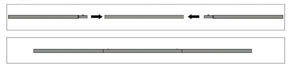
2. Slide Assembled Tube through the opening in the top of the Rolbak Net Header.
