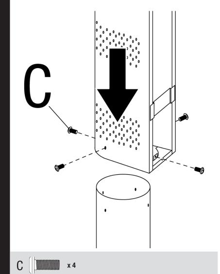
Attach Engine Assembly/Post
